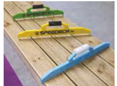
This handy jig from Speedeck enables you to get the spacing right every time on your decking projects
